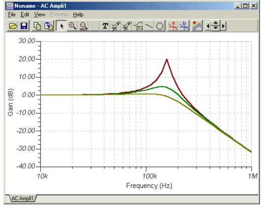
To determine which value of the stepped parameter is associated with a curve, move the cursor over the curve and read the corresponding value in the line at the bottom of the screen. You can also use the Legend and Auto label buttons in the diagram window to show the corresponding stepped values. Refer to the diagram below.
