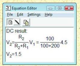
One of the most intriguing and innovative features of the new Edison is that it can not only calculate voltages and currents, but also, for linear circuits, show how these results are derived or mathematically described. For example, you can learn how to use Ohm's law, how the output of a filter varies with frequency, and how the voltage of a charging capacitor varies as a function of time.
